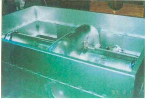
Figure 17: Barrel polishing of KEKB crab cavity [53].
