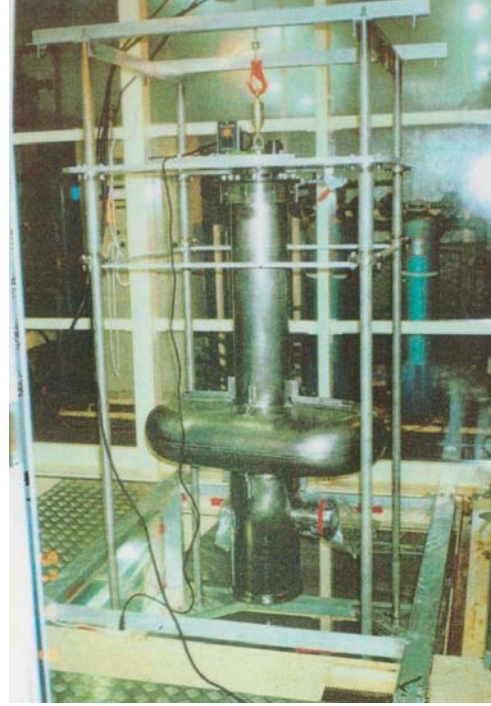
Figure 19: High-pressure water rinsing by 80-bar ultra-pure water of KEKB crab cavity [53].
