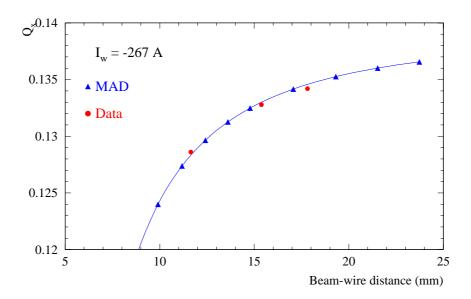
Figure 5: Observation and MAD prediction for dependence of the vertical tune on the beam-wire distance. For the data, the measured distance is corrected for the expected bias due to the wire kick.
