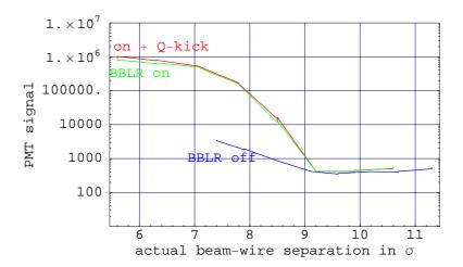
Figure 7: PMT losses versus beam-wire separation
