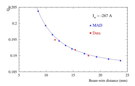
Figure 4: Observation and MAD prediction for dependence of the horizontal tune on the beam-wire distance. For the data, the measured distance is corrected for the expected bias due to the wire kick.
