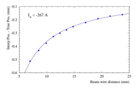
Figure 2: Simulated biais of the extrapolated beam position as a function of the true beam-wire distance for a wire current of -267 A at 55 GeV/c
