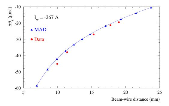
Figure 3: The observed closed orbit kick is compared to the expected kick (for a nominal wire position) as a function of the distance inferred from the beam position monitors and corrected for the bias evaluated from MAD.
