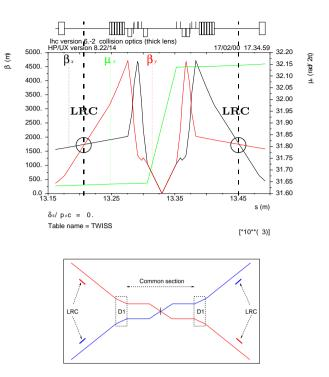
Figure 2: Twiss parameters in IR5 and schematic positions of the correctors for a horizontal crossing.
