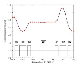
Figure 1: Beam separation in the crossing angle  $(\pm 150 \ \mu rad)$  plane of IP1 in  $\sigma$ 's
