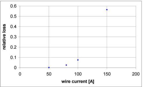
constant 6 mm distance between beam and wire center ~ 4.3 $\sigma$  at 37 GeV/c
