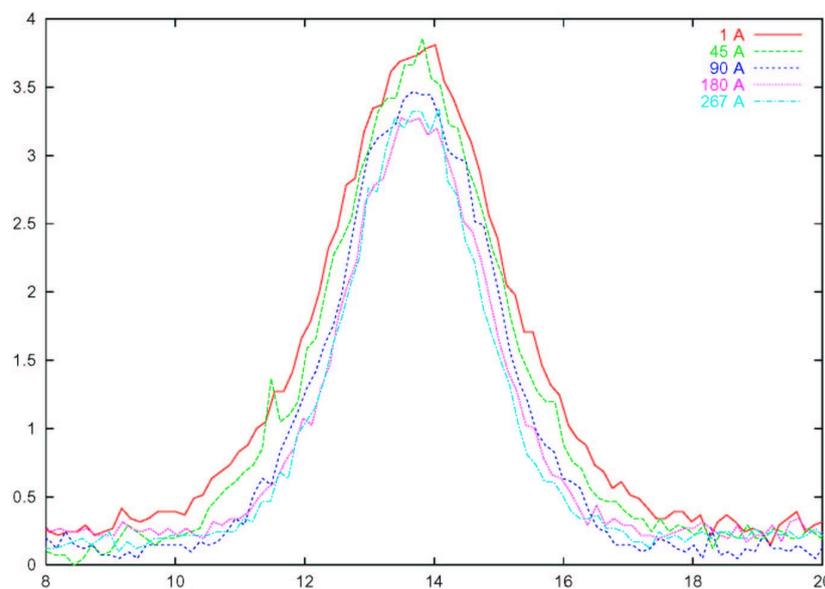
Figure 5: Vertical wire-scanner profiles obtained for different wire excitations; bump amplitude was  $-8.2$  mm, and the estimated distance between beam and center of the wire 12.1 mm.
