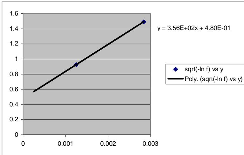
The square root of the lost beam fraction versus scraper position. The zero intersection should give the actual center of the beam.
