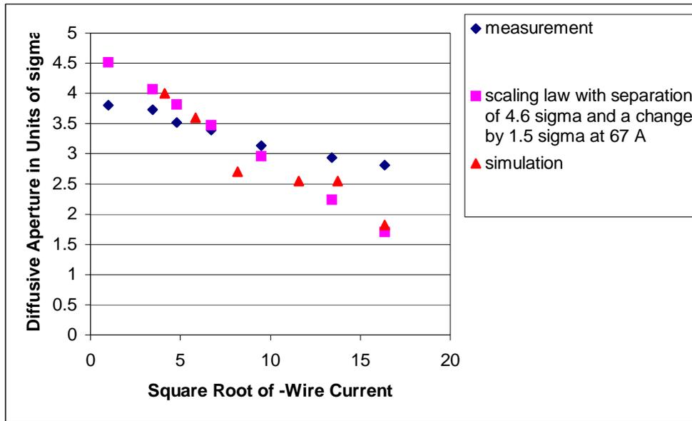
Figure 4: Diffusive aperture as a function of the square root of the wire excitation, according to (1) a rough estimate from the wire profile measurement (using the scale factor 5 obtained from a wire scan after scraping), (2) simple scaling law, and (3) weak-strong simulation.
