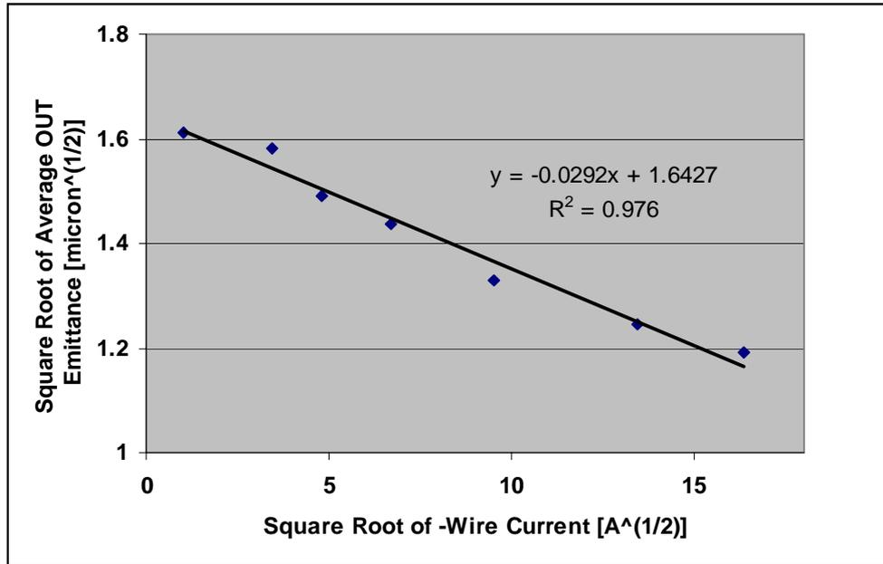
Figure 3: Square root of average OUT emittance as a function of the square root of the wire excitation.
