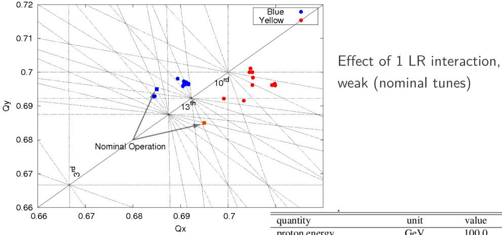
Move tunes closer to  $10^{\text{th}}$  order + octupoles ( $\Delta Q \sim 5 \times 10^{-4}$ )
