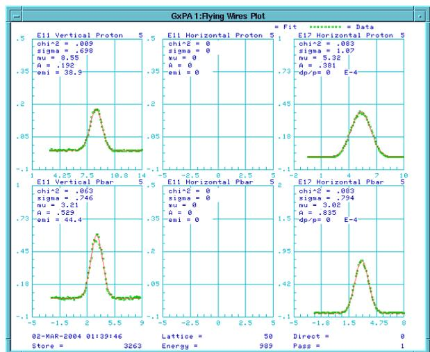
Figure 36: Flying wire scan for pbar bunch 5 before starting after TEL scan on pbars, 01:46:01.
