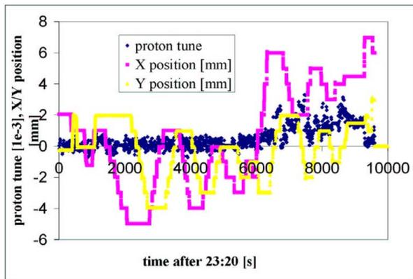
Figure 7: Variation in horizontal proton tune from 1.7-GHz Schottky monitor in units of  $10^{-3}$  measured on the three excited bunches P6, P18 and P30 as a function of time, together with the horizontal and vertical TEL position changes.
