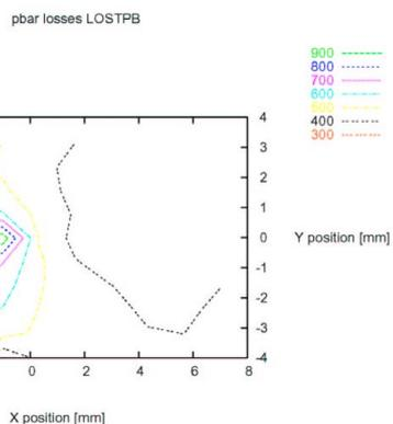
Figure 22: Contour plot of pbar losses as a function of transverse TEL positions, for all pbar bunches. Pbar beam appears to be at  $-2$  mm, 0 mm.
