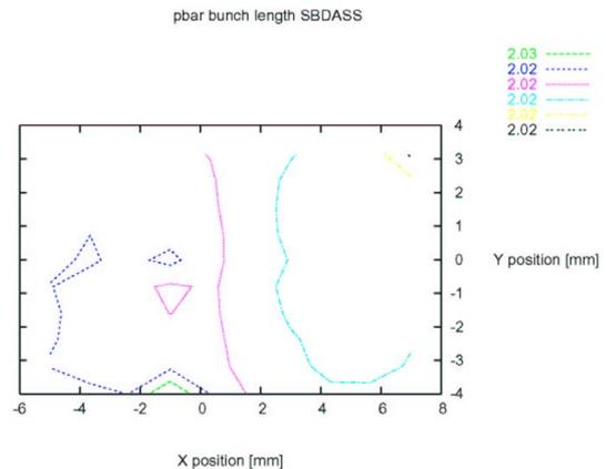
Figure 31: Contour plot of pbar bunch length as a function of transverse TEL positions, for all pbar bunches.
