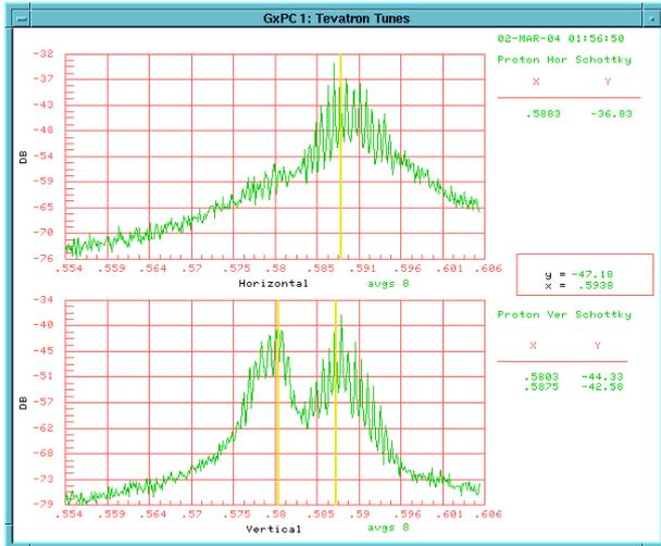
Figure 46: Horizontal and vertical spectrum from old Schottky monitor, with TEL at +5 mm, +2 mm from starting point.
