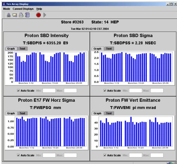
Figure 28: Proton intensity, bunch length and transverse sizes for all proton bunches. The bunches affected by the TEL, e. g., P4, P5, and P6 (the TEL pulse is too long to excite a single bunch, but in total spans about 3 bunches, with maximum amplitude at P6), show a decrease in intensity and a decrease in bunch length.
