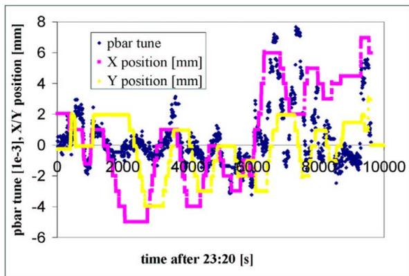
Figure 6: Variation in horizontal pbar tune from 1.7-GHz Schottky monitor in units of  $10^{-3}$  measured on the three excited bunches A5, A17 and A29 as a function of time, together with the horizontal and vertical TEL position..
