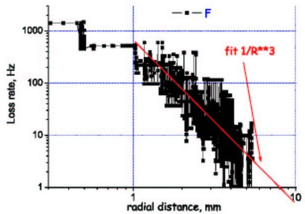
Figure 27: Antiproton loss rate as a function of TEL distance, exhibiting an inverse cubic dependence.
