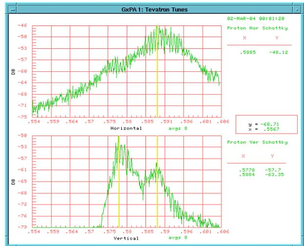
Figure 43: Horizontal and vertical spectrum from old Schottky monitor, with TEL at -7 mm, -1 mm from starting point.
