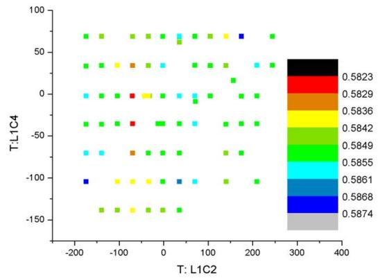
Figure 14: Pbar tune as a function of TEL corrector settings, computed by a tedious JAVA script.
