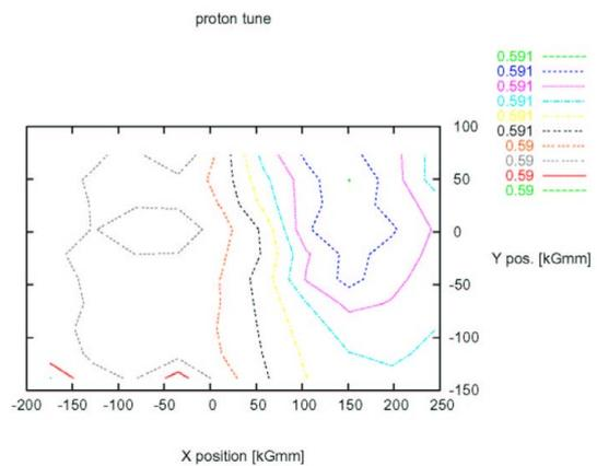
Figure 9: Contour plot of proton tune variation as a function of transverse TEL positions, for proton bunches P6, P18, and P30. Protons could be at location  $150, 50$ .
