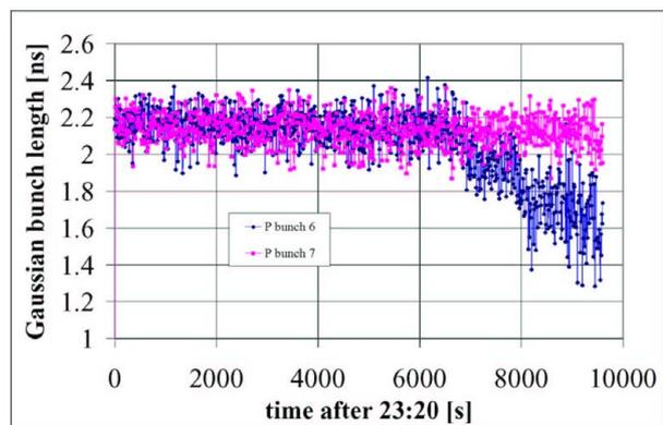
Figure 32: Bunch length from BDS Gaussian fit as a function of time for proton bunches P6 and P7. The bunch P6 which interacts with the TEL is shaved longitudinally.
