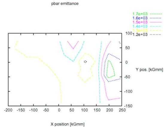
Figure 18: Contour plot of pbar emittance variation as a function of transverse TEL positions, for pbar bunches A5, A17, and A29. Pbar signal is largest when TEL is near the proton beam.
