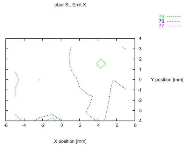
Figure 39: Contour plot of horizontal pbar emittance from SL monitor as a function of transverse TEL positions, for all pbar bunches.
