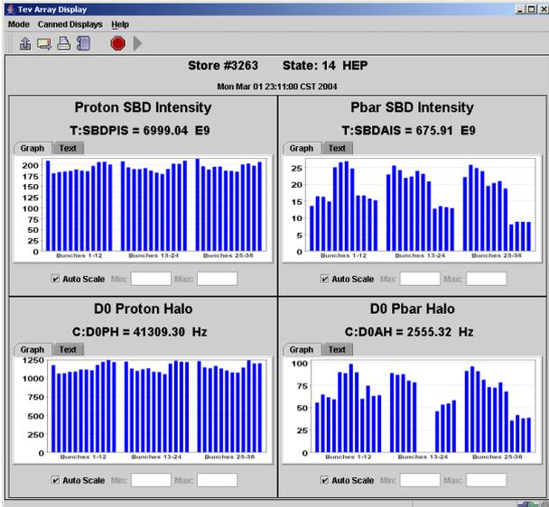
Figure 4: Proton and pbar intensities and losses after the rf trip, at 23:11:57.
