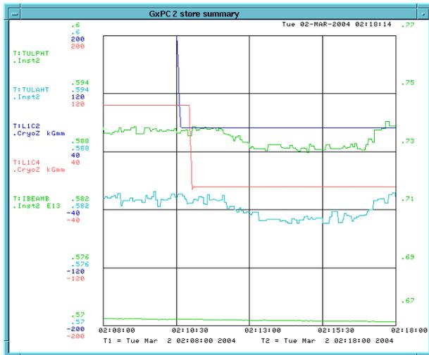
Figure 15: Response of 1.7-GHz Schottky tune fitter to a change in the horizontal base tune for protons and pbars by  $-0.002$  units.
