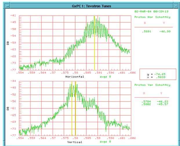
Figure 44: Horizontal and vertical spectrum from old Schottky monitor, with TEL at -2 mm, -2 mm from starting point.
