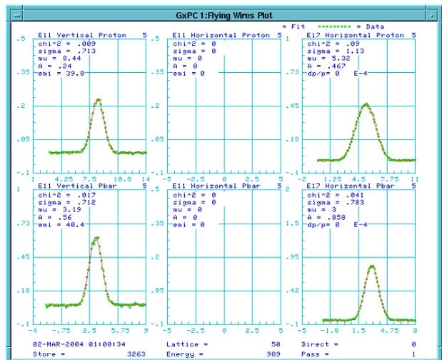
Figure 35: Flying wire scan for pbar bunch 5 before starting after TEL scan on pbars, 01:03:01.
