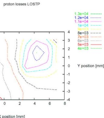
Figure 21: Contour plot of proton losses as a function of transverse TEL positions, for all proton bunches. Proton beam appears to be at location 4.5, 1.5 mm.
