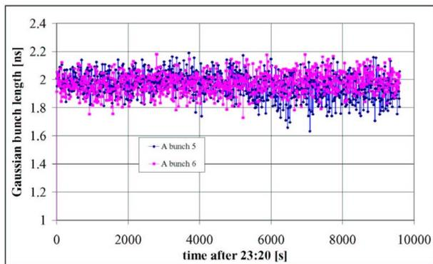
Figure 33: Bunch length from BDS Gaussian fit as a function of time for pbar bunches A5 and A6. The length of bunch A5 which interacts with the TEL does not change noticeably.
