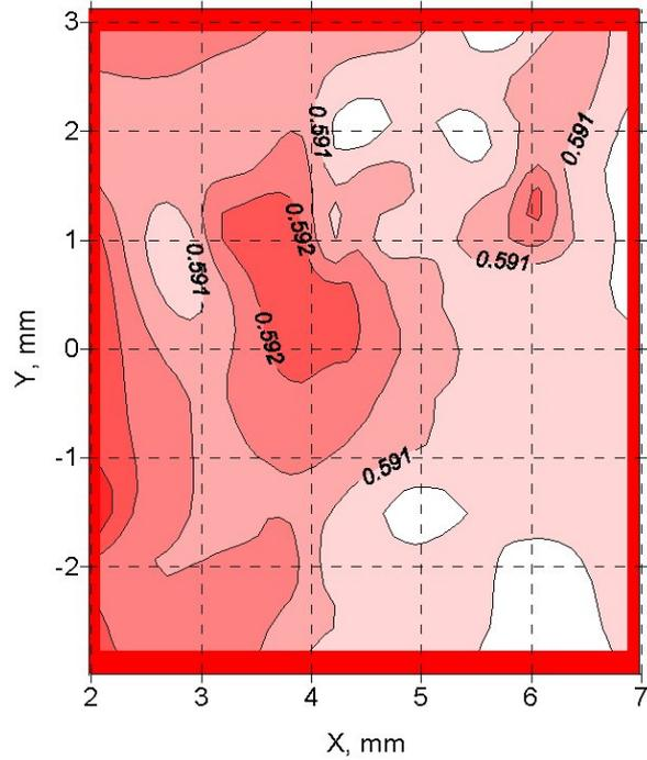
Figure 13: Proton tune as a function of TEL position.
