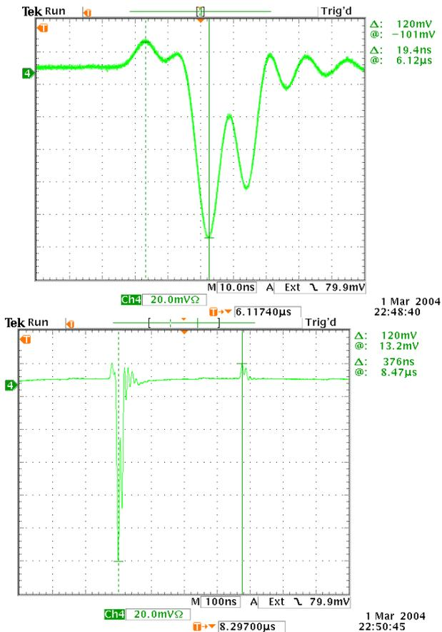
Figure 1: Top graph shows a typical proton signal at the TEL together with that of the nearest pbar bunch. The separation is about 19.4 ns. The bottom graph illustrates the distance between the last proton bunch and the last pbar bunch in the train. It is about 376ns, 20 RF buckets.
