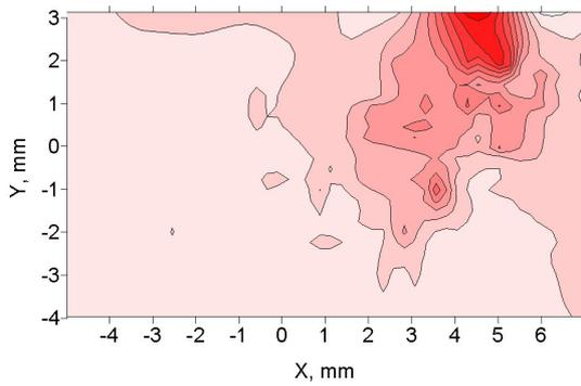
Figure 25: Contour plot of proton losses vs. TEL position.
