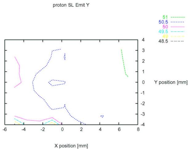
Figure 38: Contour plot of vertical proton emittance from SL monitor as a function of transverse TEL positions, for all proton bunches.
