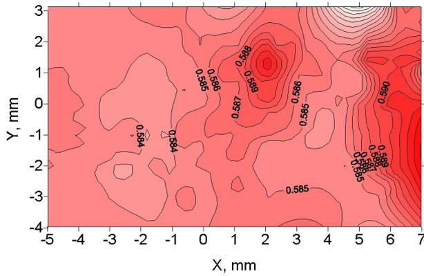
Figure 11: Pbar tune as a function of TEL position over a wider horizontal range.
