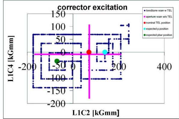
Figure 5: Corrector excitation pattern during the MD. Visible are the aperture scan without TEL in pink in the form of a cross and the 2-dimensional grid scan with TEL. Also indicated are the expected nominal positions of TEL, protons, and pbars, respectively, as (very roughly) extrapolated from the upstream TEL-BPM readings. The solenoid field is 35 kG and therefore 35 kGmm correspond to 1 mm displacement on either axis. L1C2 controls the horizontal electron position, L1C4 the vertical.
