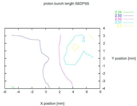
Figure 30: Contour plot of proton bunch length as a function of transverse TEL positions, for all proton bunches.
