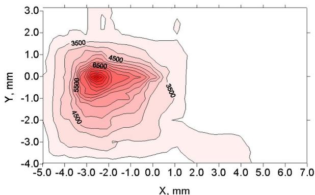
Figure 23: Contour plot of all pbar losses vs. TEL position.
