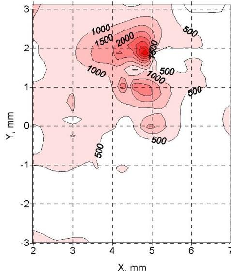
Figure 26: Contour plot of proton losses vs. TEL position after better synchronization.
