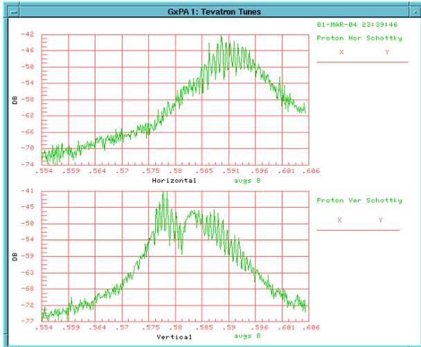
Figure 41: Horizontal and vertical spectrum from old Schottky monitor, with TEL at -1 mm, +2 mm from starting point.
