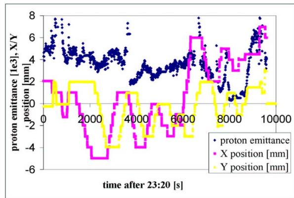
Figure 17: Variation in horizontal proton “emittance” from 1.7-GHz Schottky monitor in (uncalibrated) units of  $10^3$  measured on the three excited bunches P6, P18 and P30 as a function of time, together with the horizontal and vertical TEL position changes.
