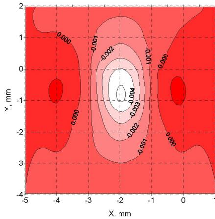
Figure 12: Predicted tune shift for pencil pbar beam.
