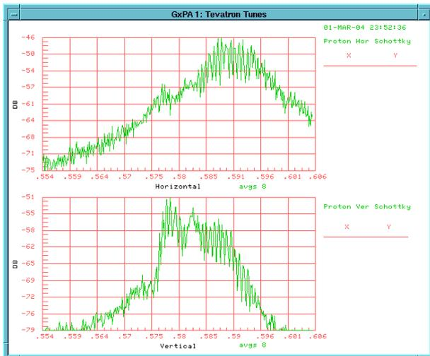
Figure 42: Horizontal and vertical spectrum from old Schottky monitor, with TEL at -6 mm, +2 mm from starting point.
