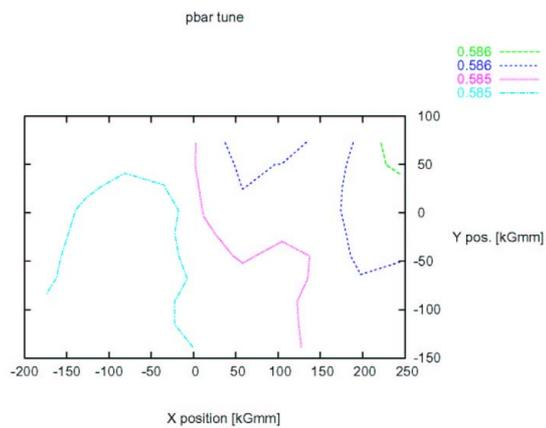
Figure 8: Contour plot of pbar tune variation as a function of transverse TEL positions, for pbar bunches A5, P17, and A29. Pbars could be at location  $-100, -50$ ?
