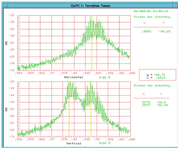
Figure 45: Horizontal and vertical spectrum from old Schottky monitor, with TEL at +4 mm, 0 mm from starting point.
