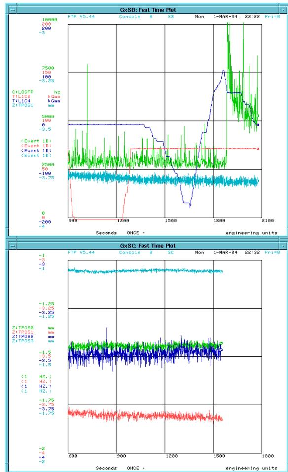
Figure 3: Proton loss rates plus TEL corrector settings L1C2 and L1C4 and 1 proton beam position reading (top picture); several beam position readings (bottom picture), during aperture scan without TEL electron beam. Changing TEL correctors by +3(4) mm did not increase proton losses. The peak at the end was due to a trip of pbar RF station 5. Beam orbit in TPOSx changed by not more than 10 microns.
