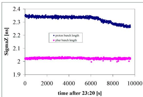
Figure 29: Bunch length from BDS Gaussian fit as a function of time, averaged over all proton and pbar bunches. The proton beam is shaved longitudinally
