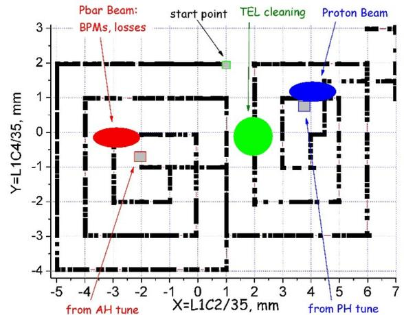
Figure 47: Summary of TEL position scan. Beam sizes are approximately to scale.
