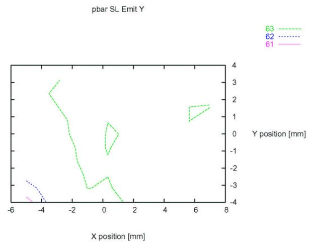
Figure 40: Contour plot of vertical pbar emittance from SL monitor as a function of transverse TEL positions, for all pbar bunches.
