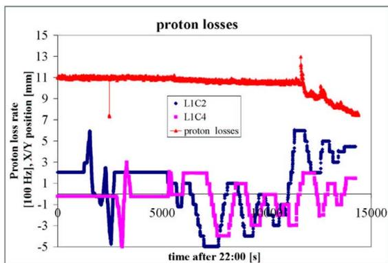
Figure 20: Average loss rate in proton bunches P6, P18 and P30 as a function of time, together with the the TEL horizontal and vertical position.
