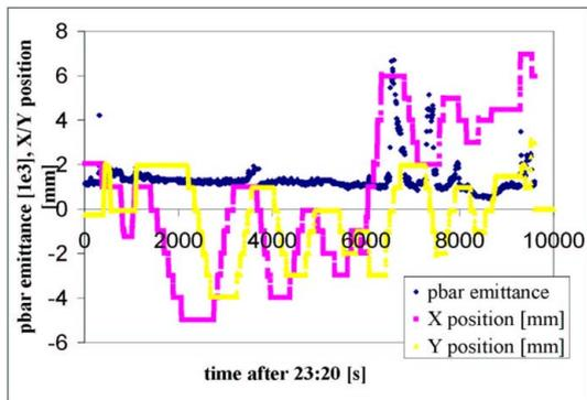
Figure 16: Variation in horizontal pbar “emittance” from 1.7-GHz Schottky monitor in (uncalibrated) units of  $10^3$  measured on the three excited bunches A5, A17 and A29 as a function of time, together with the horizontal and vertical TEL position changes.
